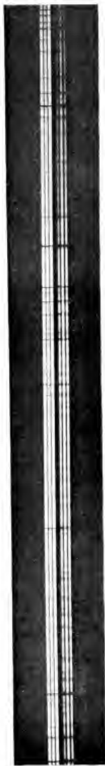
FIG. 15.—Rotation Spectrum Photographed without and with Air-Currents in the Spectrograph.
