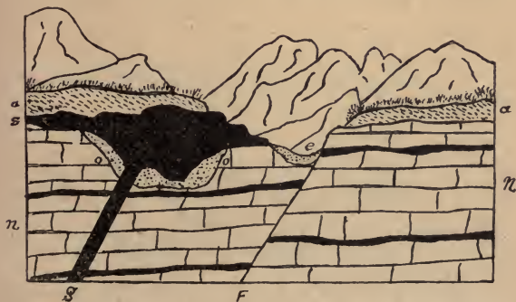
This section shows an old river bed covered by a trap overflow, which forced the river to take a new course, along the line of a "fault." A A —Earth. E —New Channel. O O —covered gold-bearing gravel. N N —The formation. F —Fault. S S —Trap overflow.
