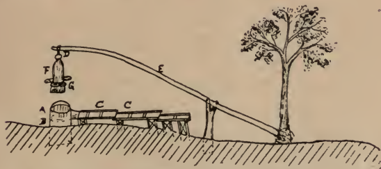
A - Cushion bars. B. - Hollowed block. C.—Sluites. D.—Chain-hook. E.—Spring pole. F.—Dolly. G.—Iron shoe.
