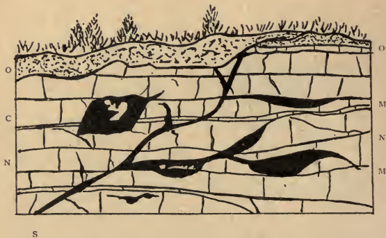
The above section shows a common occurrence of Galena Veins. oo—Surface Clay. NN—Limestone. M—main bodies of ore. c—a Pocket. s—the Lode.
