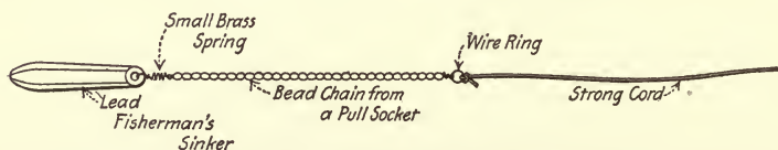
FIG. 130.—Mouse with chain inserted.
