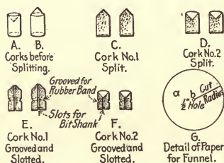
FIG. 94.—Parts of holder for dirt-catcher.
