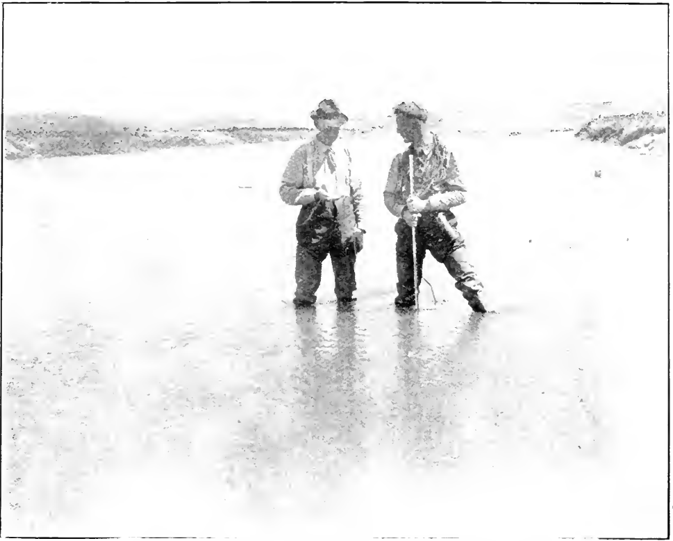
Measuring the Velocity with a Current Meter by Wading.
