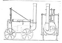
and side view of this machine. This locomotive engine, which in many of its leading features was essentially the same as those now in use, drew at its first trial as many wagons as carried ten tons of bra-iron, with a considerable number of persons, and travelled at the rate of five miles an hour. The "tender," carrying a supply of fuel and water, and a small force-pump, worked by the machine itself, maintained the requisite quantity of water in the boiler.
