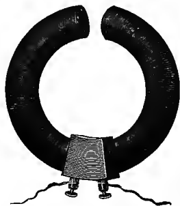
FIG. 29.—A nearly closed magnetic circuit.
