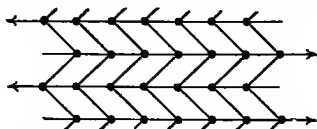
FIG. 7A. Closer representation of electric displacement or shear. Cords alternately representing positive and negative electricity. Cf. also Fig. 46.
