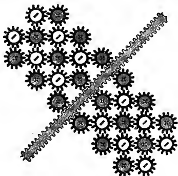
FIG. 39.—A provisional representation of a current surrounded by dielectric medium, either propelling or being propelled. Section through the wire. Compare Fig. 30, B.
