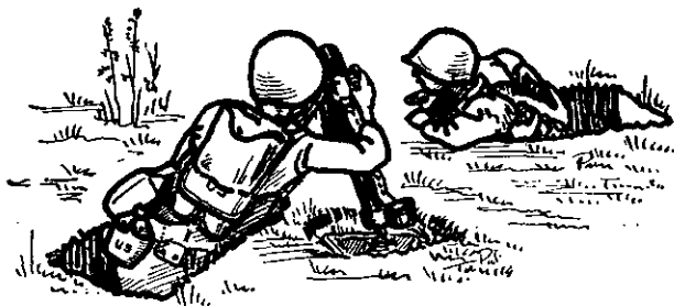
FIGURE 35.—Emplacement for 60-mm mortar with standing type one-man foxholes. (Standing type one-man foxhole for observer is also prepared. His location is within voice range of the mortar emplacement.)
