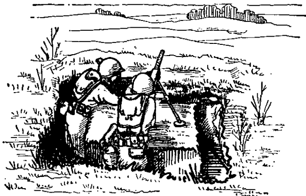
FIGURE 34.—Light machine-gun emplacement. (The gun platform is approximately 6 inches below ground level. Spoil is used to form a low parapet around the emplacement, or it is scattered; sod is used on top of the parapet.)
